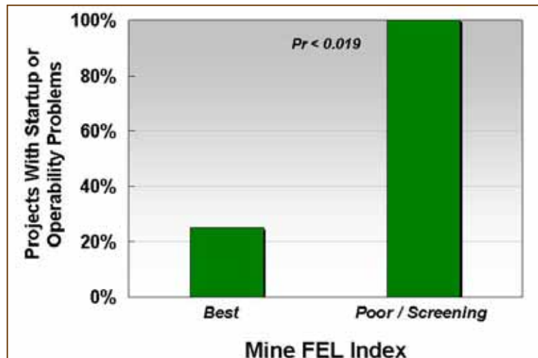
Figure 3. Better Mine Definition Drives Reduced Startup/Operability Problems
